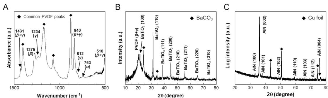
**Figure 2.** Characterization results of the films. (A) FTIR and (B) XRD of PVDF+BTO film. (C) XRD of AlN on Cu foil. FTIR: Fourier-transform infrared spectroscopy; PVDF: polyvinylidene fluoride; BTO: BaTiO<sub>3</sub>; AlN: aluminum nitride.
