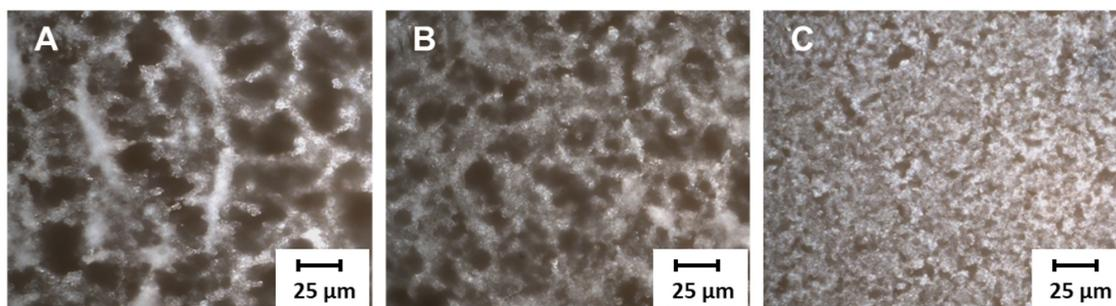
**Figure 3.** Optical microscope images of PVDF films with (A) 5 wt.%; (B) 10 wt.%; and (C) 30 wt.% BTO-NPs. PVDF: Polyvinylidene fluoride; BTO-NP: BaTiO<sub>3</sub> nanoparticle.
