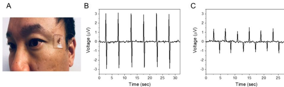
**Figure 7.** Sensing of eye blinking and eyeball movement. (A) Image of the sensor attached to the temple area. Voltage output characteristics of (B) eye blinking and (C) lateral eyeball movement.
