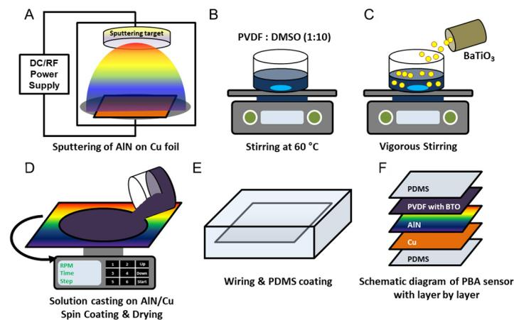
**Figure 1.** Illustration of the steps used to prepare the PBA sensor. (A) AlN sputtering deposition on Cu foil; (B) PVDF solution; (C) BTO-NP dispersion in PVDF; (D) PVDF+BTO-NP solution casting on AlN/Cu foil then spin coating and drying of PVDF+BTO-NP film; (E) wiring and PDMS sealing; and (F) Schematic diagram of PBA sensor. PBA: PVDF+BTO-NP/AlN; AlN: aluminum nitride; BTO-NP: BaTiO<sub>3</sub> nanoparticle; PVDF: polyvinylidene fluoride.
