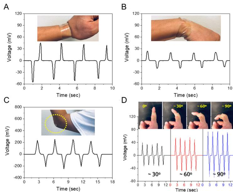
**Figure 8.** The piezoelectric PBA sensor characteristics from several joint motions. Voltage outputs of different types of wrist movements: (A) upward and (B) downward bending. Monitoring the bending amplitude of joints with the help of a Band-Aid; (C) elbow; and (D) finger with various bending angles. Inset photos represent the position where the PBA sensor was attached. PBA: PVDF+BTO-NP/AIN.
