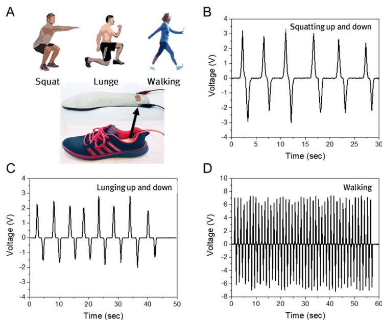
**Figure 9.** The piezoelectric performance of pressure sensing. (A) Illustration of practices and photographs of PBA sensor located in the insole of a shoe. The voltage output of pressure arising from (B) squatting; (C) lunging; and (D) walking. PBA: PVDF+BTO-NP/AIN.
