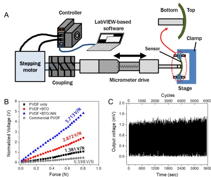
**Figure 5.** Characterization of electromechanical conversion of different piezoelectric films. (A) Schematic illustration of a custom-made piezoelectric test station; (B) electromechanical conversion in terms of applied force vs. output voltage of films normalized with 10- $\mu\text{m}$  thickness; and (C) changes in output voltage over 5000 cycles using a repeated force of 0.2 N.
