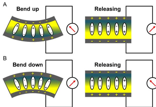
**Figure 4.** Sensing mechanism of piezoelectric sensor with (A) bend-up and (B) bend-down conditions followed by releasing to the initial state before bending.
