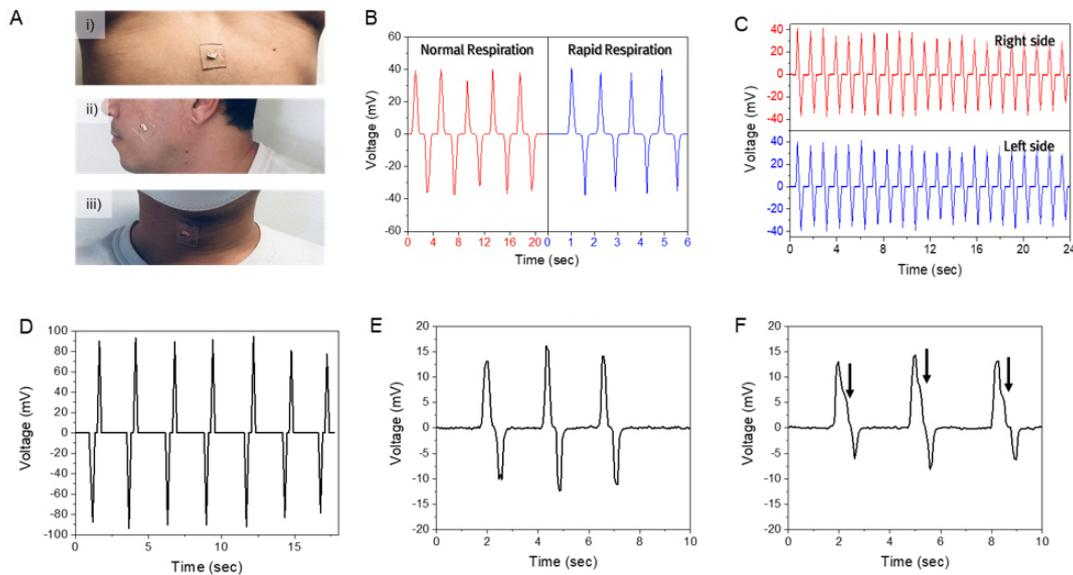
**Figure 6.** Piezoelectric pressure sensor for muscle motion monitoring. (A) Photographs of the sensor positions such as (i) diaphragm; (ii) jaw; and (iii) neck. The output voltages from (B) normal and rapid respiration, (C) chewing; and (D) swallowing. The output voltages from vocal stimulus (E) “Hi” and (F) “Houston”. The arrows indicate the second syllable.
