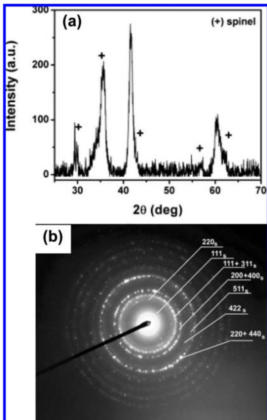
**Figure 2.** (a) XRD and (b) TEM-SAED patterns of polycrystalline iron–manganese oxide samples. Rings with  $s$  subscripts arise from the spinel  $\text{MnFe}_2\text{O}_4$  phase, and the other rings arise from  $\text{Fe}_{1-x}\text{Mn}_x\text{O}$  ( $0 < x < 1$ ) phases.
