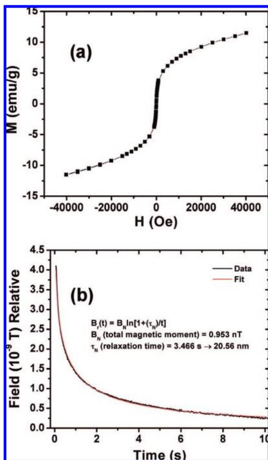
**Figure 4.** (a) Hysteresis loop of superparamagnetic iron–manganese oxide nanoparticles at room temperature and (b) magnetic relaxation curve of iron–manganese oxide nanoparticles magnetized at a field of 2 mT. The solid curve is the corresponding Néel relaxation fit.
