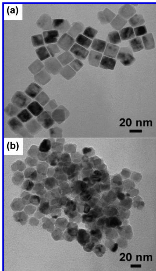
**Figure 3.** Shape variation of iron–manganese oxide nanoparticles upon variation of the ester content. Ratio of 16-heptadecenoic acid:ethyl heptadecenoate equals (a) 4:1 and (b) 1:1.
