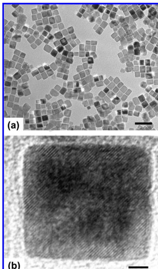
**Figure 1.** (a) Conventional bright-field (scale bar = 50 nm) and (b) HR-TEM image (scale bar = 2 nm) TEM images. The average body-centered diagonal size shown here is  $29 \pm 4$  nm. Two analogous preparations afforded identical distributions of  $33 \pm 5$  nm.
